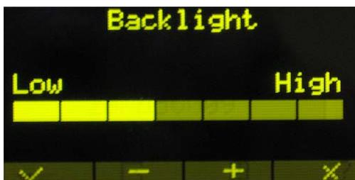
To **increase the backlight brightness level of the Keypad Buttons**, Press "+".
